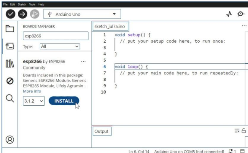
Now, go to **Tools > Board > ESP8266 Boards** and select **LOLIN(WEMOS) D1 mini (clone)** OR **LOLIN(WEMOS) D1 mini Pro**, depending on your board.
